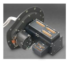
The Side-Drive Solar Array Drive Mechanism (SADM) consists of a slip ring assembly and an actuator coupled by a spur gear set, which, when driven by suitable drive electronics, will position the Solar Array toward the sun for maximum power and transfer the collected energy to the spacecraft power bus. The SADM unit is an integrated assembly of actuator, slip ring with integral position
